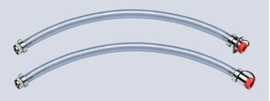
To install, simply screw the extension onto the wick oiler in place of the cover, the tube can then be shortened to any length. Fix the filling nozzle (for type 1) with 2 countersunk screws  $\emptyset$  3 mm and press in the upper tube clip. Always ensure that the flow of oil to the wick oiler is guaranteed during installation.
