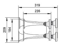
If snow caps are used, the overall length of the acoustic horns is increased by 30 mm.
