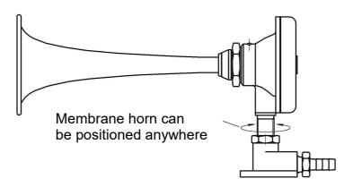
Our newly developed anodised aluminium brackets make assembly much easier. The horns can be mounted from one side and fixed in any direction. The bracket can also be combined with the elbow connections Art. no. 2568.14. To reduce the installation height, the threaded sleeve can be shortened by 15 mm (avoid chips in membrane housing).
